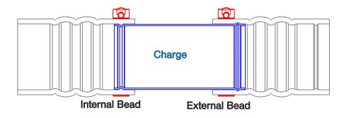
For charge pipes with internal bead rolls a silicone boot with an internal bead should be used. Internal bead should be positioned in the internal bead roll. Clamp should be placed directly over bead roll and tightened.
